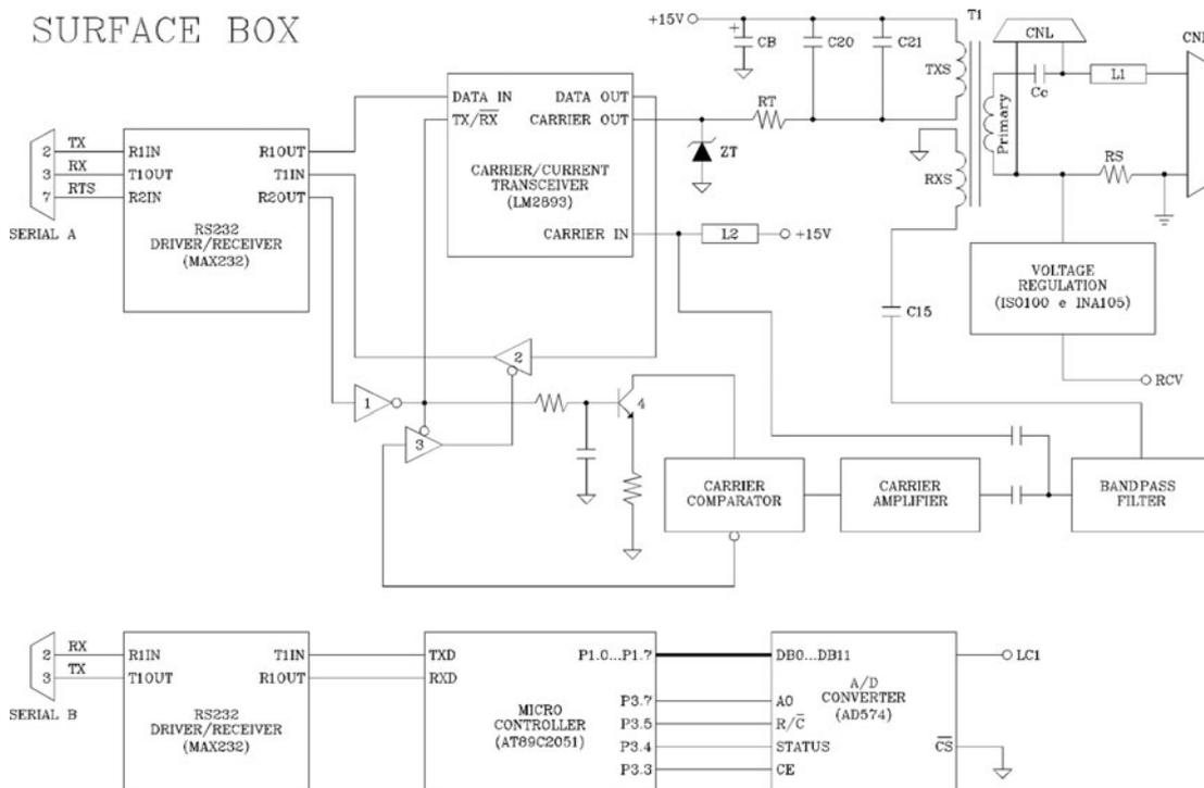
**Fig. 3.** Surface box outline, including two principal electronic circuits: the first for communication with the BHS, with the LM2893 modem and voltage regulation; the second for the connection to the load cell. Through two serial circuits we have transmission of the remote data to the console program.
