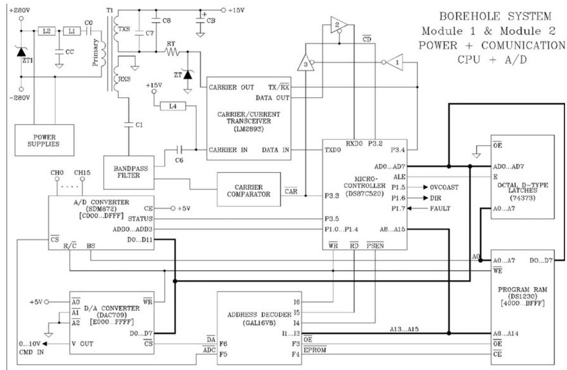
**Fig. 4.** Modules 1 and 2 outline, including the first two BHS modules, the communication/power module with the LM2893 modem and the power regulation section, and the CPU module that collects and sends remote data. The LVDT circuit is not represented; it is commercially made by H.F. Jensen.
