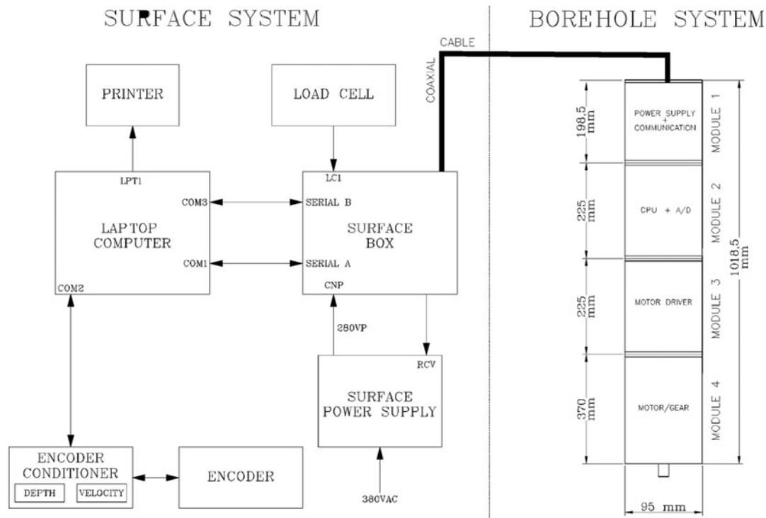
**Fig. 2.** Overall system, including physical components of the electronic control system: the computer used for the console program; the load cell; the encoder; and the surface box that interfaces all these systems and is connected, through the drilling cable, to the BHS.
