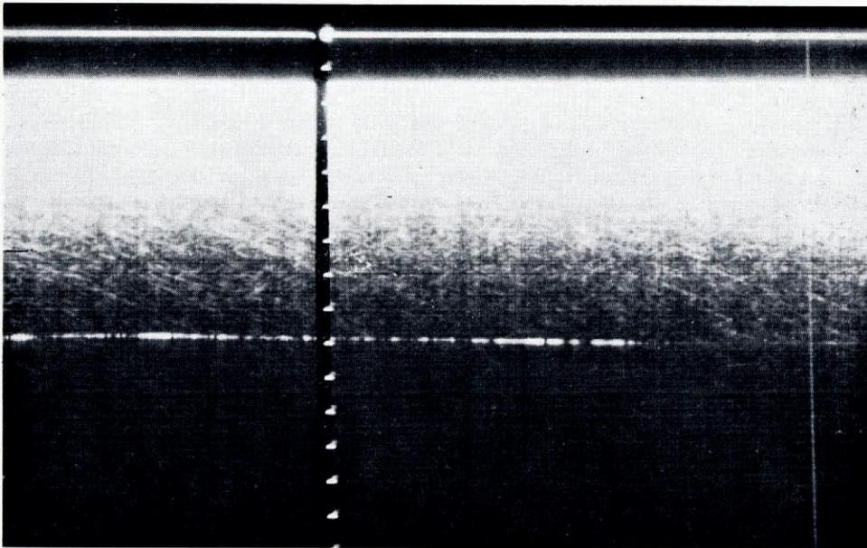
*Fig. 5. The echo from a position where the ice is thought to be at the pressure-melting point, without the formation of a definite "lake".*
