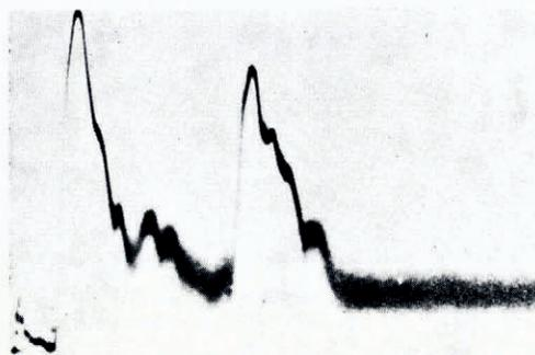
Fig. 6. An example of an "A-scope" trace. The horizontal axis covers about 800 m of ice depth: the vertical axis is a logarithmic scale of echo strength, with a range of some 60 dB. The trace is initiated at the left-hand end of the scale, and the peak near the centre represents the bottom echo.
