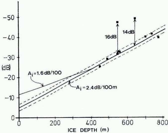
Fig. 8. Echo strength versus ice depth on the Devon Island ice cap. The power is expressed in terms of the total attenuation due to absorption in ice ( $A_i$ ) and reflection losses at the bedrock. The dotted lines represent the standard error arising from the linear regression.
