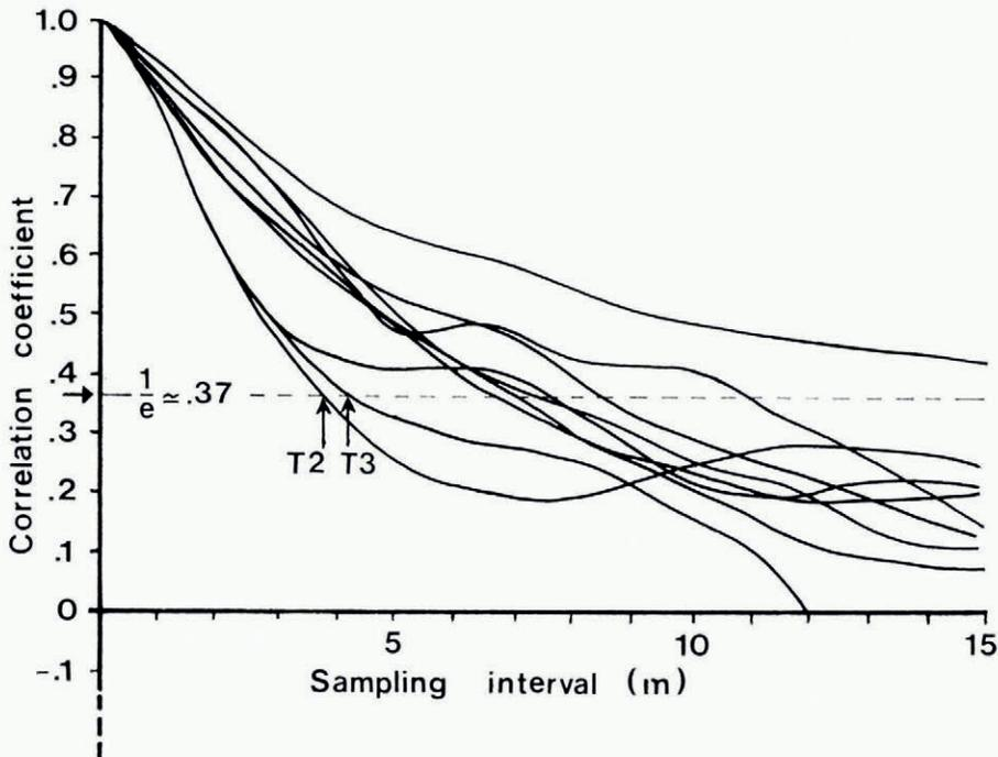
Fig. 10. Autocorrelation functions for nine sets of echo strength measurements at 1 m intervals.
