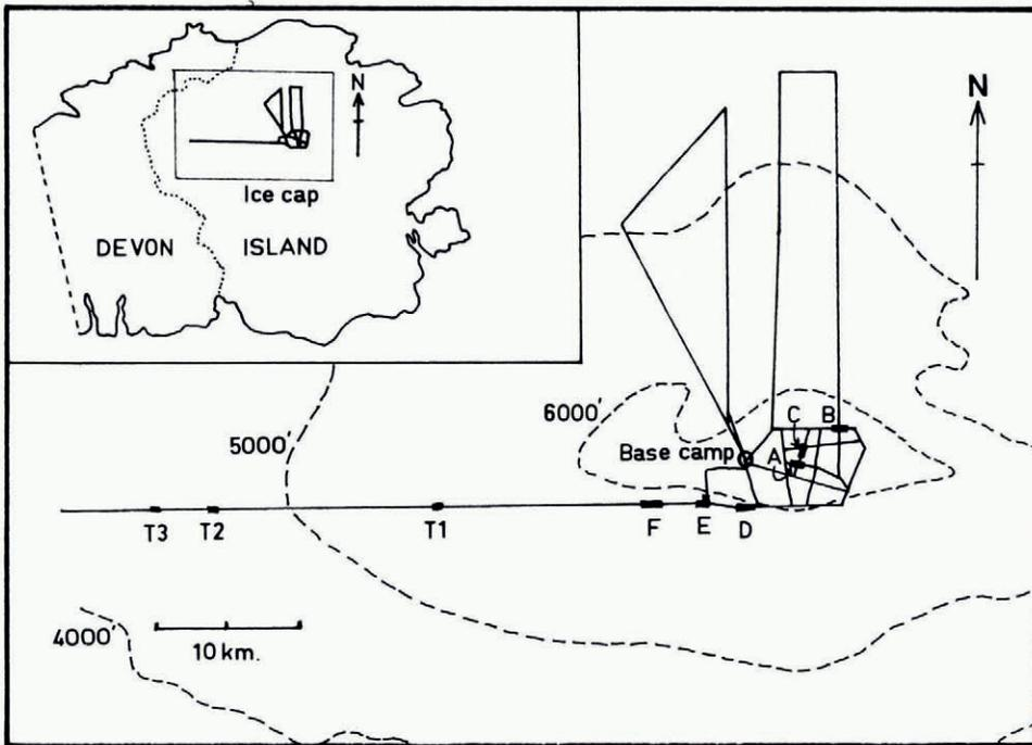
Fig. 7. The inset map shows the eastern end of Devon Island, the ice cap covering most of the area to the east of the dotted line. The positions of the survey lines, and of the nine sets of closely spaced strength measurements, can be seen at larger scale in the main part of the figure. Contours are in feet; 5000 ft = 1520 m.
