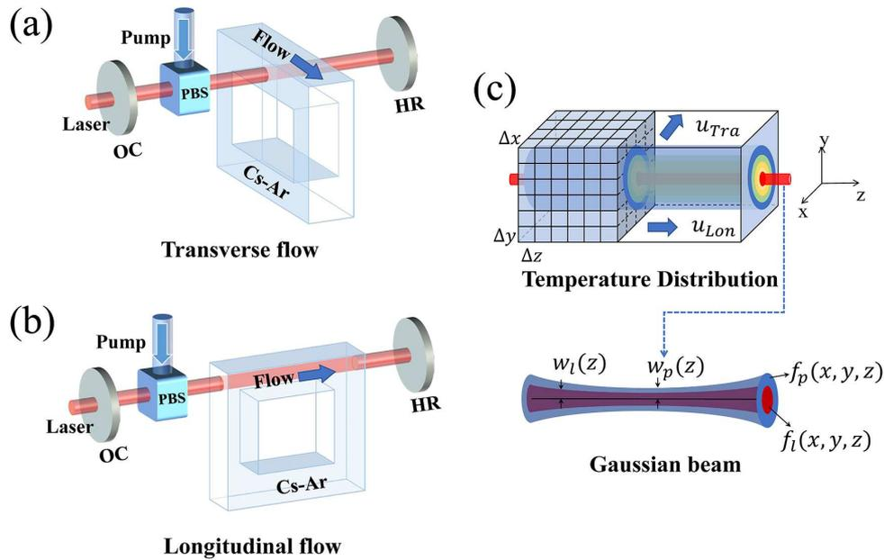
Figure 1. Sketch of optical systems of XPCsL.
