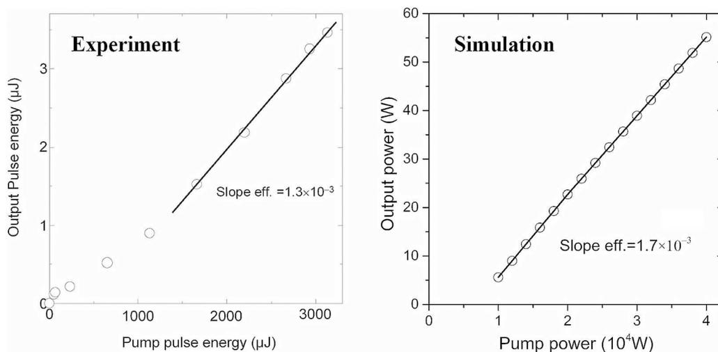
**Figure 3.** Comparison of slope efficiency between experiment<sup>[19]</sup> and simulation results.
