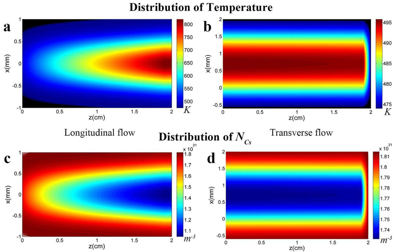
**Figure 5.** (a), (b) The temperature distribution in the  $x$ - $y$  plane at  $y = 0$  in Figures 4(a) and 4(b). (c), (d) The distribution of  $N_{Cs}$  in the  $x$ - $y$  plane at  $y = 0$  in Figures 4(a) and 4(b).
