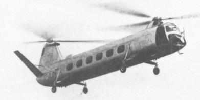
The Bristol 173 Helicopter is fitted with two Alvis Leonides Engines
