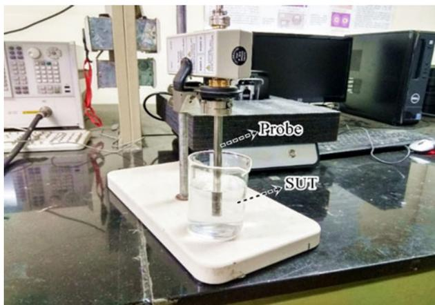
Fig. 7. Permittivity measurement setup using the dielectric probe kit (85070 E) method.
